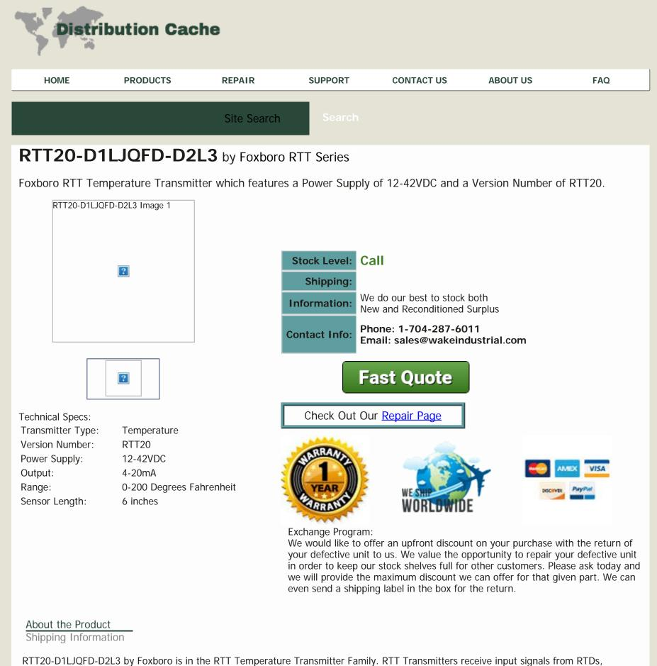
thermocouples, ohms sensors, or dc mV sources. This RTT20-D1LJQFD-D2L3 transmitter offers a 12-42VDC Power Supply and Version Number of RTT20. It also features a Transmitter Type of Temperature and an Output of 4-20mA.
