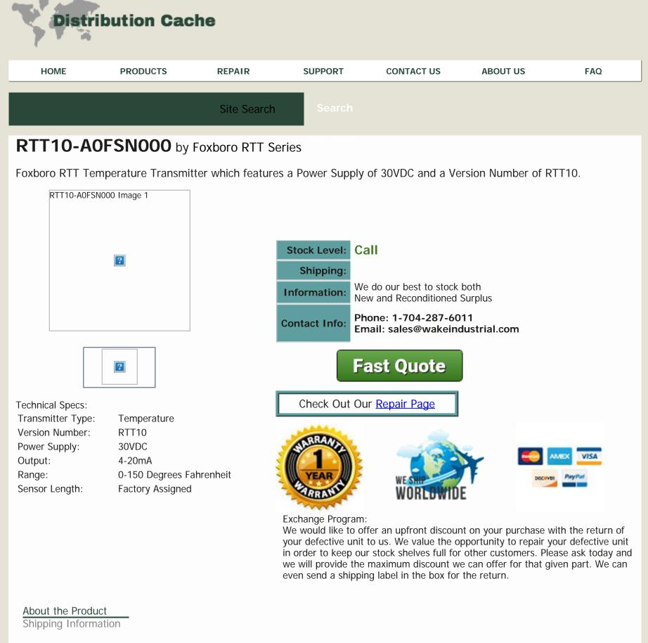
RTT10-A0FSN000 by Foxboro is in the RTT Temperature Transmitter Family. RTT Transmitters receive input signals from RTDs, thermocouples, ohms sensors, or dc mV sources. This RTT10-A0FSN000 transmitter offers a 30VDC Power Supply and Version Number of RTT10. It also features a Transmitter Type of Temperature and an Output of 4-20mA.
